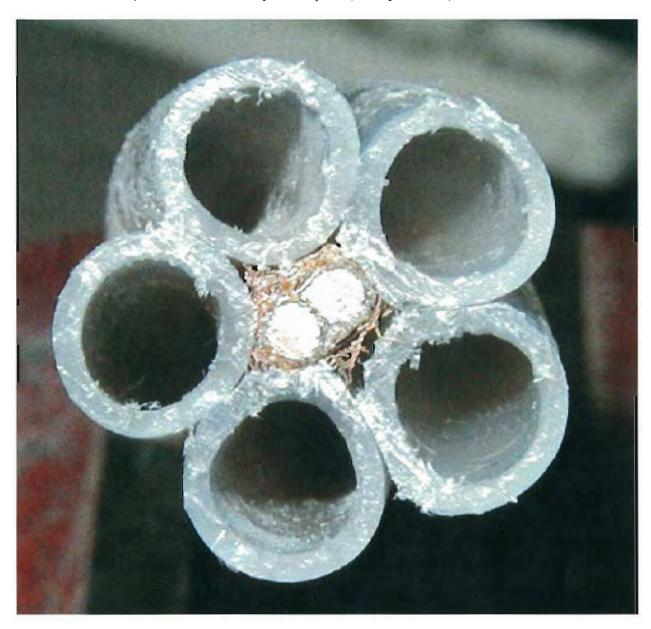
4. Umbilical Failure (Teflon tubes that carry mercury sample completely melted)
