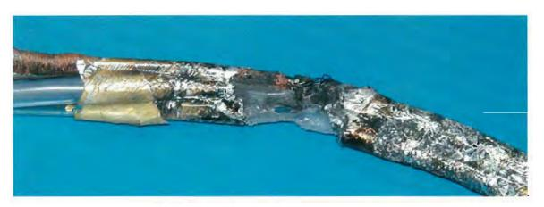
3. Umbilical Failure (Teflon tubes that carry mercury sample begin to melt)
