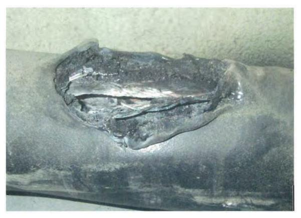
2. Umbilical Failure (Teflon tubes that carry mercury sample melted from heat trace over heating)
